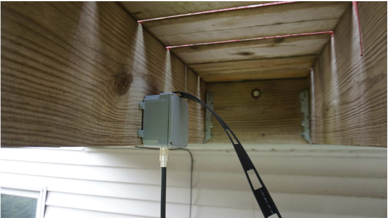
Picture of window line connecting to balun on top; coax connection on bottom. Coax goes to grounded bulkhead connector before entry into the house.
